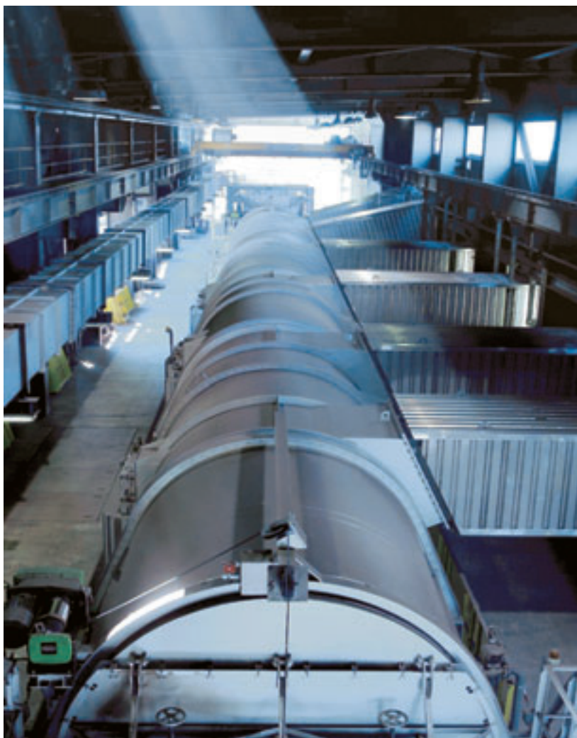
Figure 1: Hooded sinter strand with offgas recirculation ducts seen to the right
