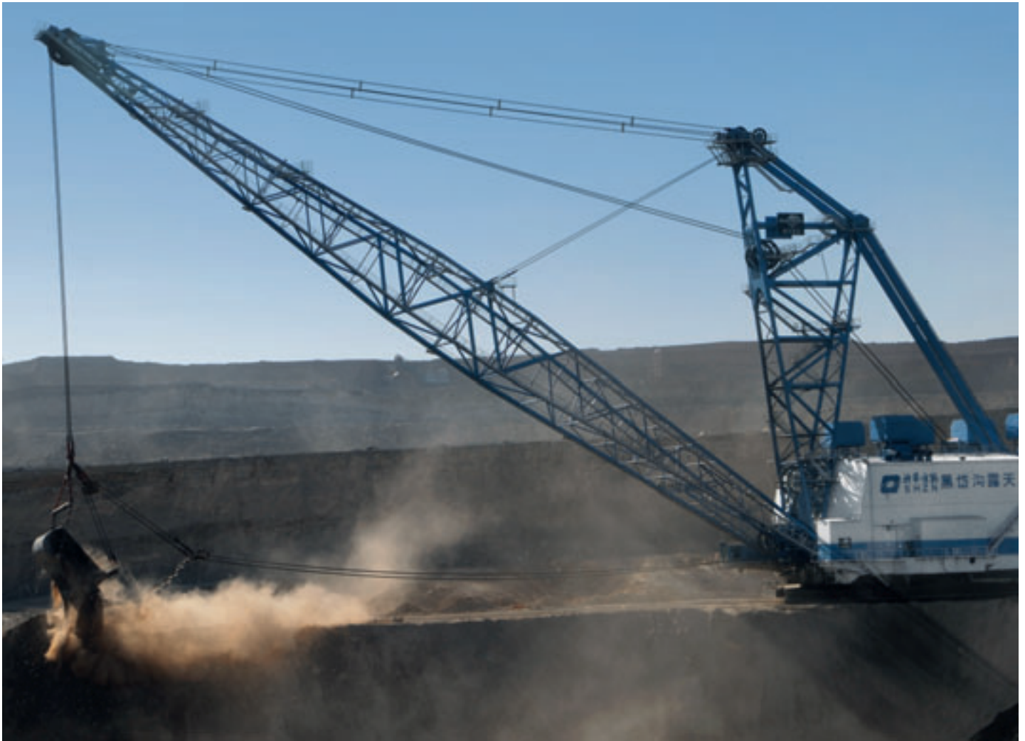
The Bucyrus excavator with the new drive system for use in the Chinese Zhungeer coal mine
