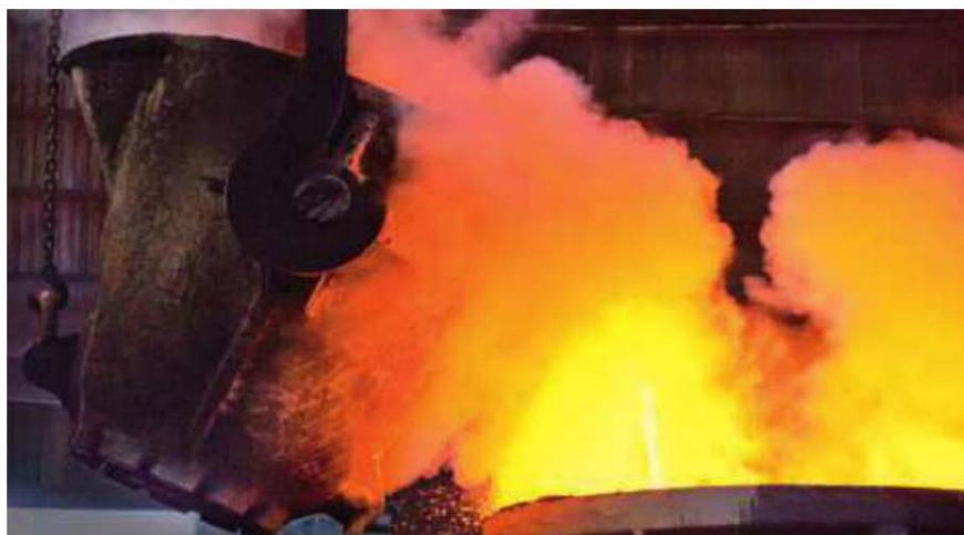
Slag from a converter is being poured to a slag pot in a workshop of the RMK's Karabashmed industrial complex located in Karabash city, Chelyabinsk region.
