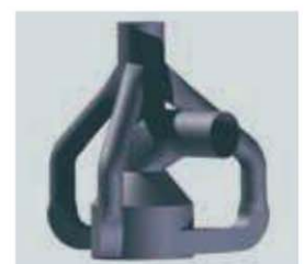
New three-inlet cyclone
