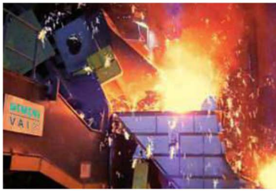
Simetal EAF hot-metal charging
