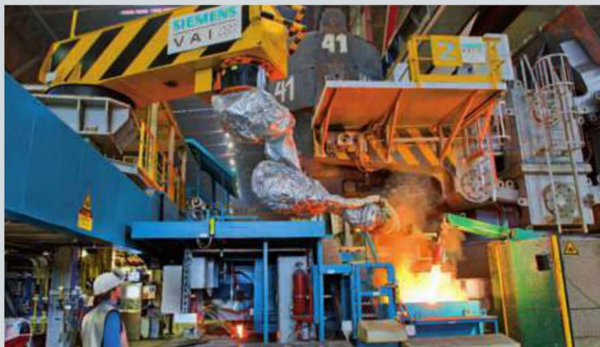
CC7 caster equipped by Siemens at voestalpine Stahl in Linz, Austria. The casting platform is automated by the LiquiRob robot systems
