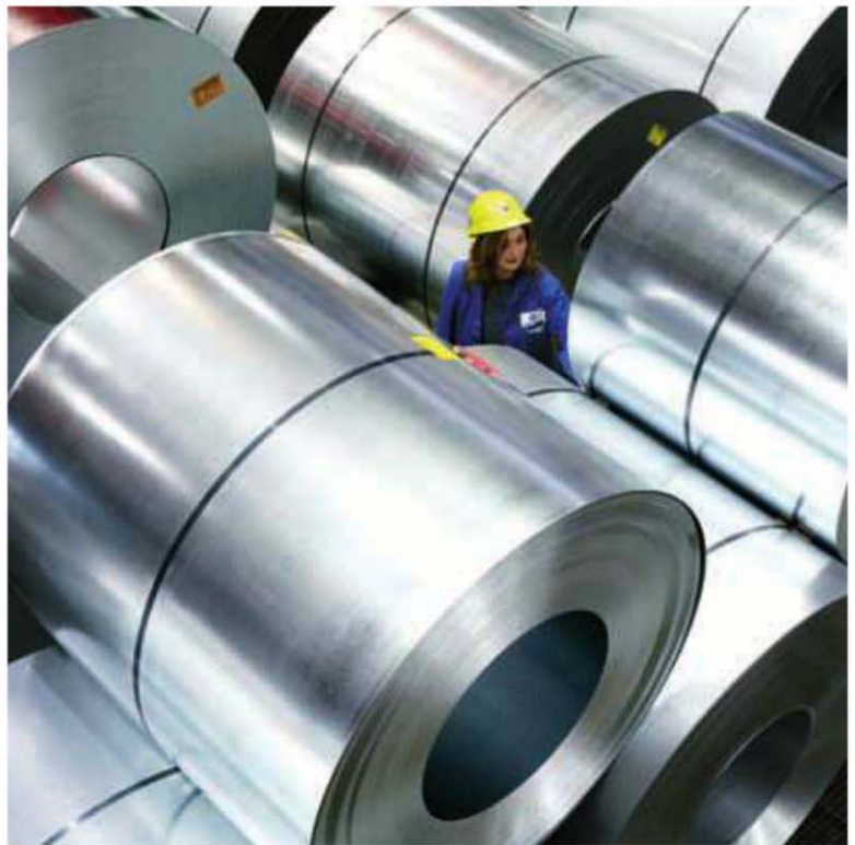
Angelika Kostall inspects steel strip fresh from the galvanizing shop at EKO Stahl, an Arcelor company
