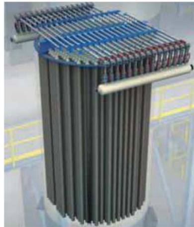
New bag-filter system for fine dust capture
