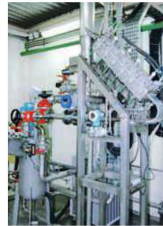
Laboratory investigations of electrolytic iron ore reduction in the Ulcwin process
