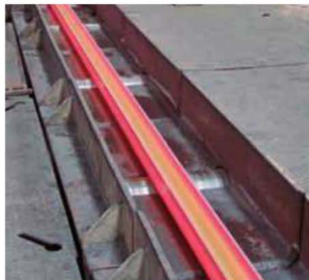
Section rolled on a Siemens rolling mill for medium-sized products
