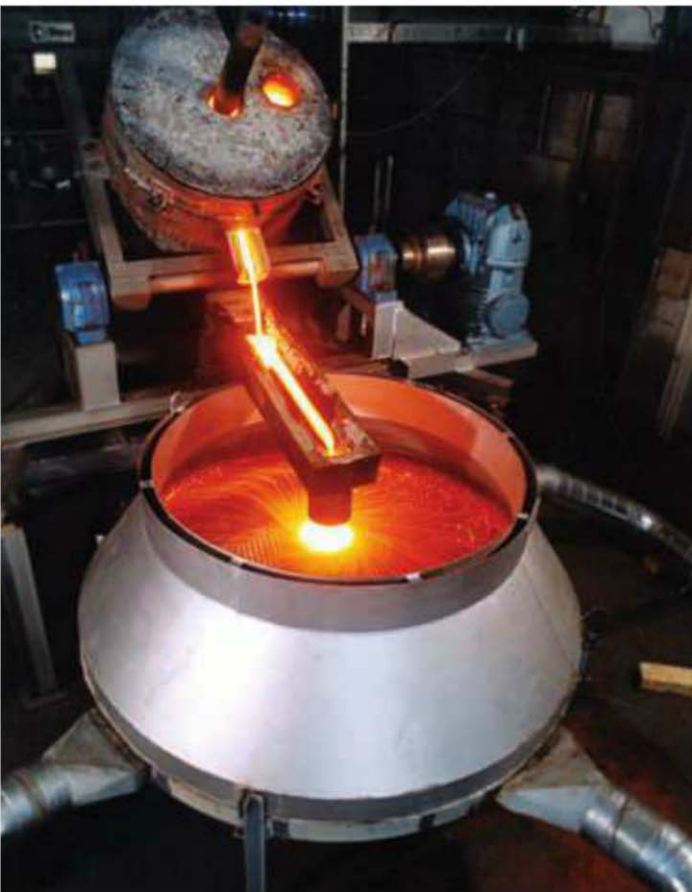
Pilot dry-slag granulator in operation
