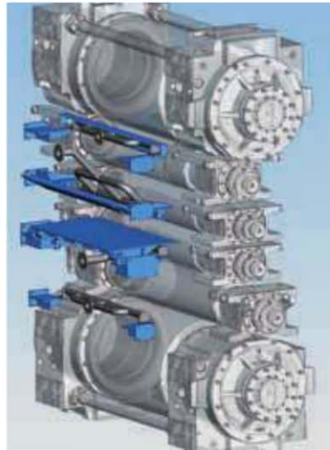
Roll-gap lubrication and strip blow-off system
