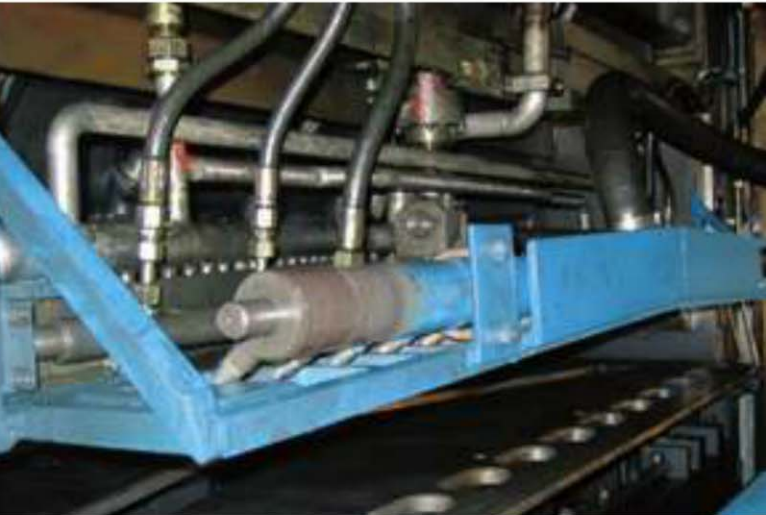
Direct application headers on entry side of the cold reversing mill at ISD Dunafer
