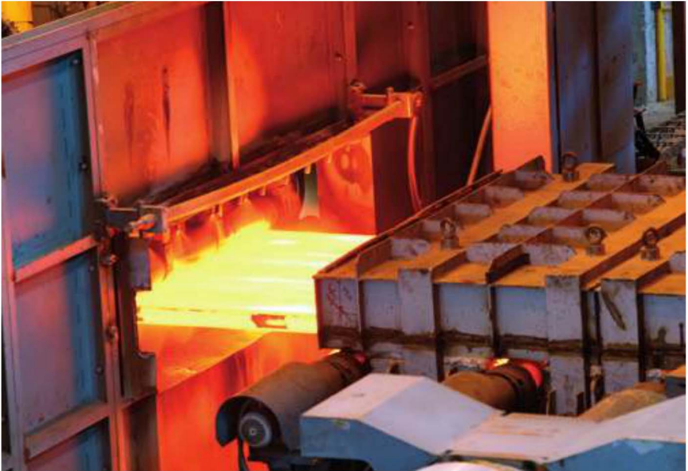
Thin slabs are produced here, and later they will be rolled in a hot mill
