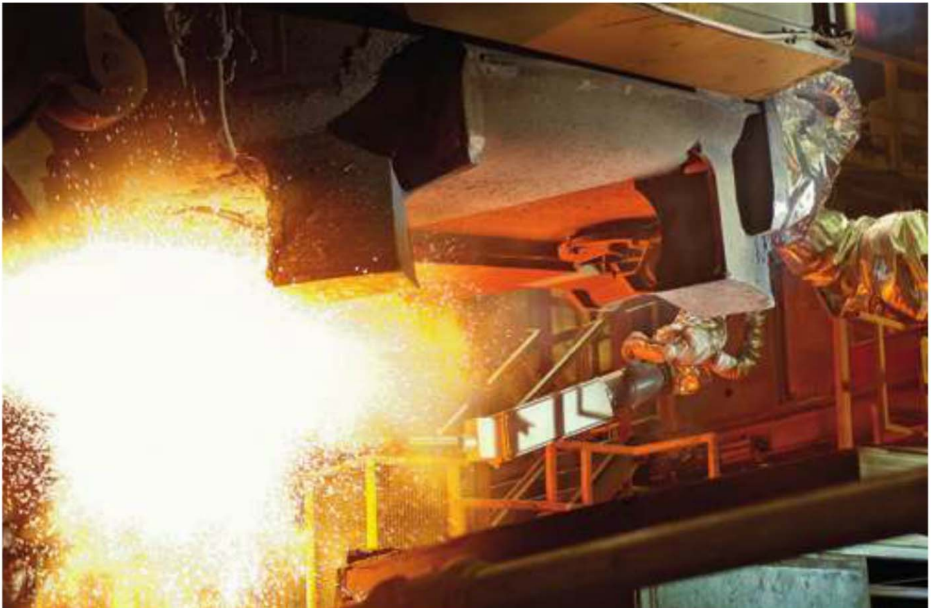
The robot system Simetal LiquiRob automates the casting platform and improves operational safety
