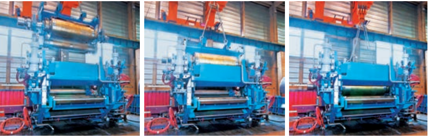
Workshop demonstration of easy insertion of the Pinch-Roll Quick-Exchange Unit into the unit housing
