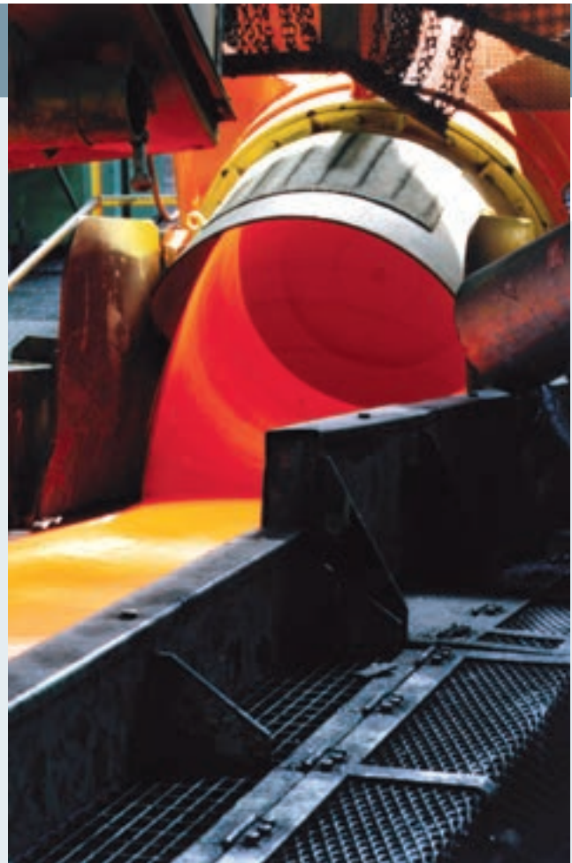
Example of a Morgan high-speed laying head for wire rod
