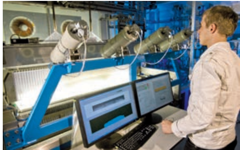
The latest spray nozzle designs are optimized in testing stands to meet the increasing requirements placed on secondary strand cooling
