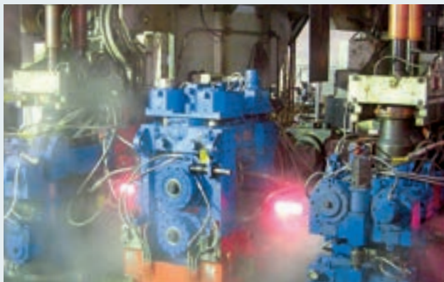
Example of a sizing train from Siemens VAI
