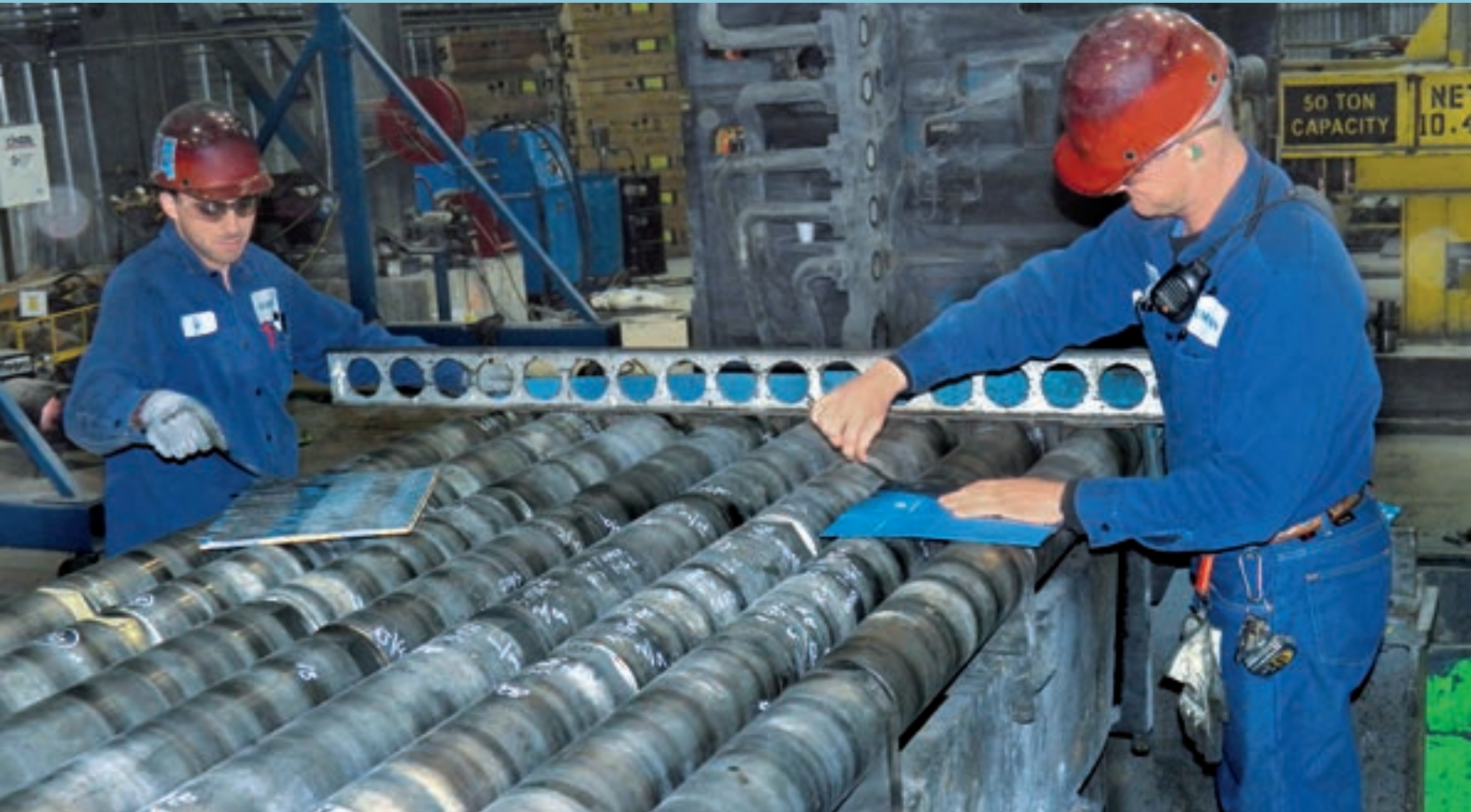
Fig. 2: Siemens VAI Columbus employees set roll heights on a caster segment
